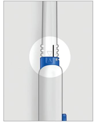
4. Firmly support the tip of the sensor holder while gently moving the blue slide forward until it covers the sensor.
